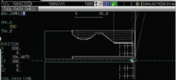
Tool path check By tool path simulation, the accurate machining cycle time is quickly obtained
