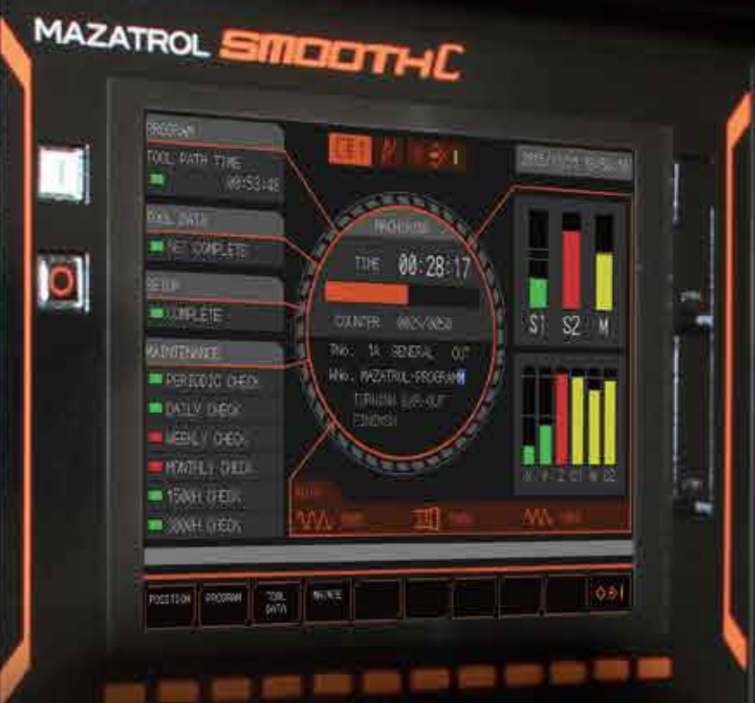
Process home screen The home screen displays overall process status in an easy to understand manner.
