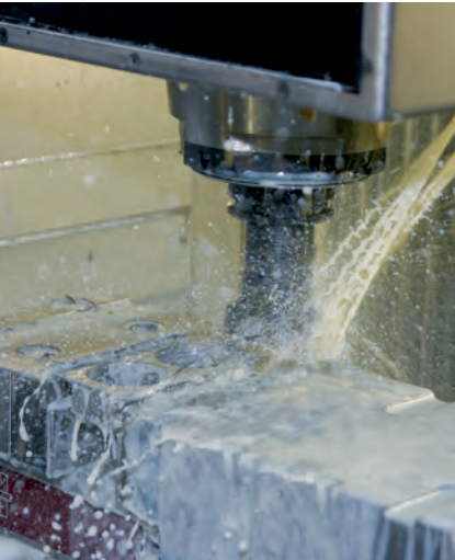
Example of Flood Coolant for cooling and lubricating when mechanically machining components.
