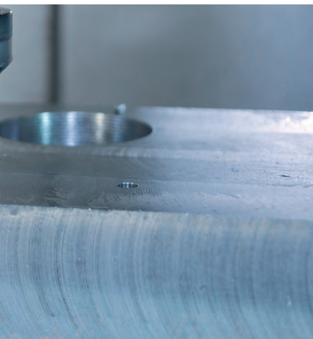
Thread Forming with the MQL 2-channel system.
